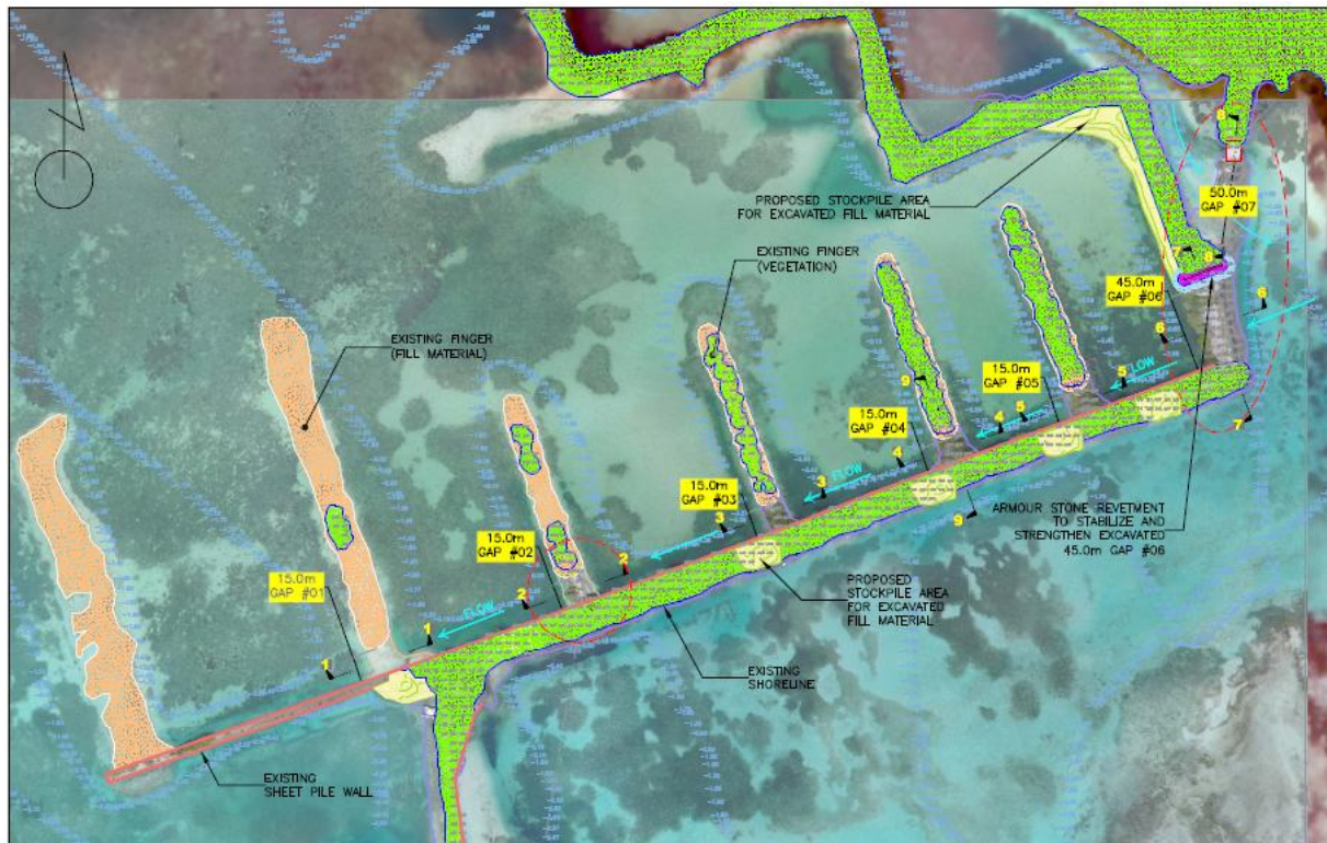
Figure 2: The engineering designs created by Smith Warner International. Gaps 1 to 5 have now been excavated thanks to funding from Philip Stephenson Foundation and the Grenadines Partnership Fund.
